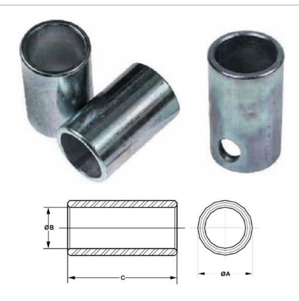
Used in the pin hole of a lift arm to allow a smaller Category pin to fit. Clear trivalent chromate plating.
